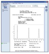
The eCord chip provides the user with QC test conditions and results on the column run by the manufacturer. The information includes mobile phases, running conditions, and analytes used to test the columns. In addition the QC results and acceptance is placed onto the column.
